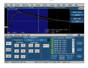
NOTE. To manually fit the waveform into the mask, select Manual Fit in the Control pane. You can manually fit only one waveform at a time into the mask.
